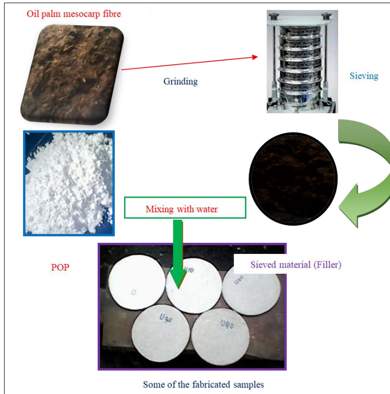
Figure 1 Pictorial illustration of the samples' fabrication processes
