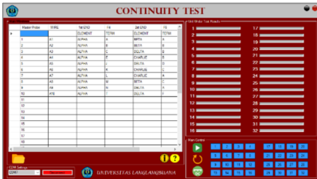
Figure 9 Main window with wirelist data
