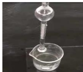
Figure 28 Determination of Surface tension using Stalagmometer
