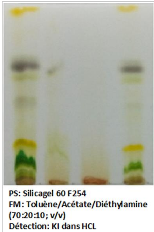
Figure 5 TLC chromatogram of methanolic extracts of the two plants studied at 366 nm
