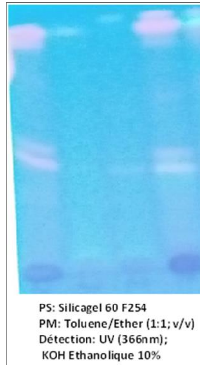
Figure 6 TLC chromatogram of methanolic extracts of the two plants studied at 366 nm
